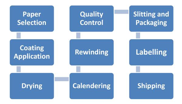
The manufacturing process of sublimation heat transfer paper rolls involves several key steps, focusing on the creation of a high-quality paper that is capable of transferring vibrant, durable images onto fabrics or other materials through a sublimation process. Below is an outline of the typical manufacturing process:
